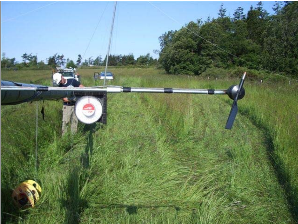
Figure 2.3 – Wind Direction Sensor at 30 Meters
