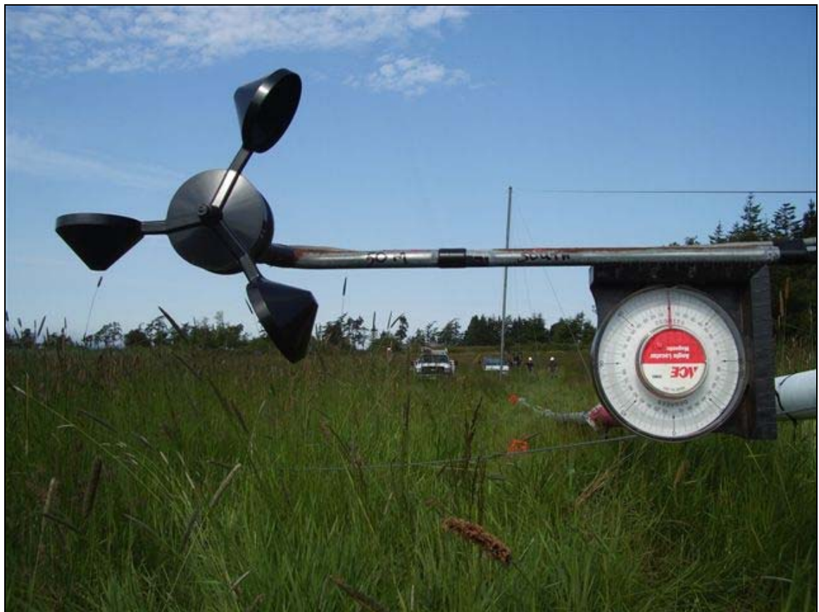
Figure 2.2 – Wind Speed Sensor at 50 Meters and 180 Degrees
